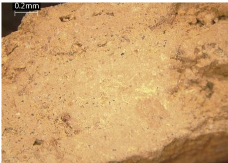
3. A thin section of a vessel fired in a kiln at 670°C. 8x magnification Leica Stereomicroscope EZ4.
