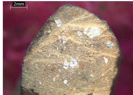
8. Renče clay with admixed calcite, Sample 12. 8x magnification Leica Stereomicroscope EZ4.
