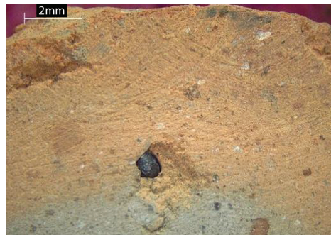
6. Renče clay, fired at 800°C, Sample 7. 8x magnification Leica Stereomicroscope EZ4.
