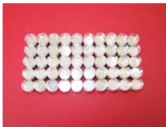
Figure 1. Titanium specimens were surrounded by a sellotape.
