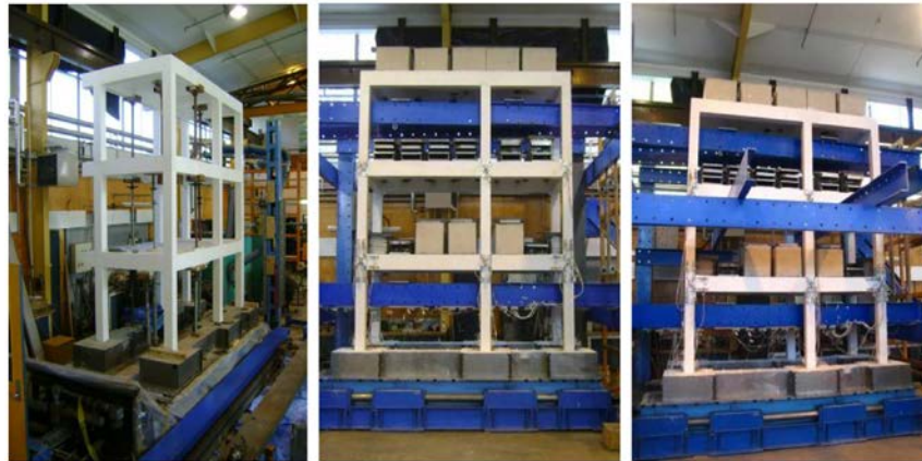
(a) 1:2.5 scale three storey two bays by one bay deficient RC model tested by Quintana et al. [10]
