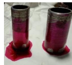
Fig. 8. Specimen during LPT on penetrant application
