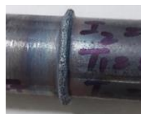
Fig. 9. MIAB Weld Sample with reinforcement
