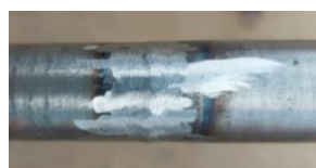
Fig. 10. MIAB Weld Sample without the reinforcement
