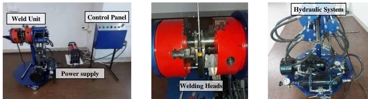
Fig. 7. Experimental Setup: a) machine setup; b) welding heads; c) hydraulic system
