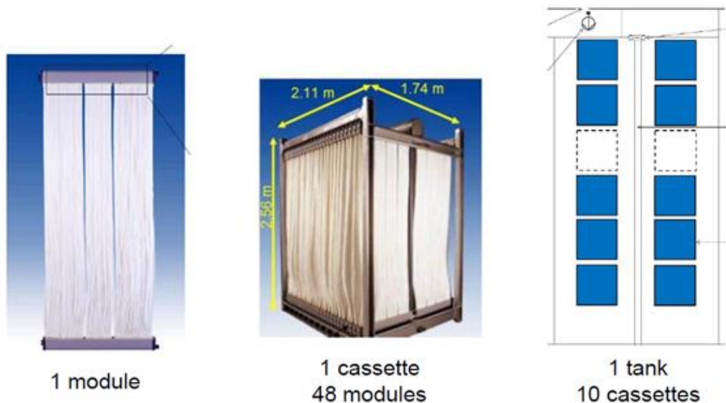
Fig. 6.8: Module, cassettes, and single MBR tank
