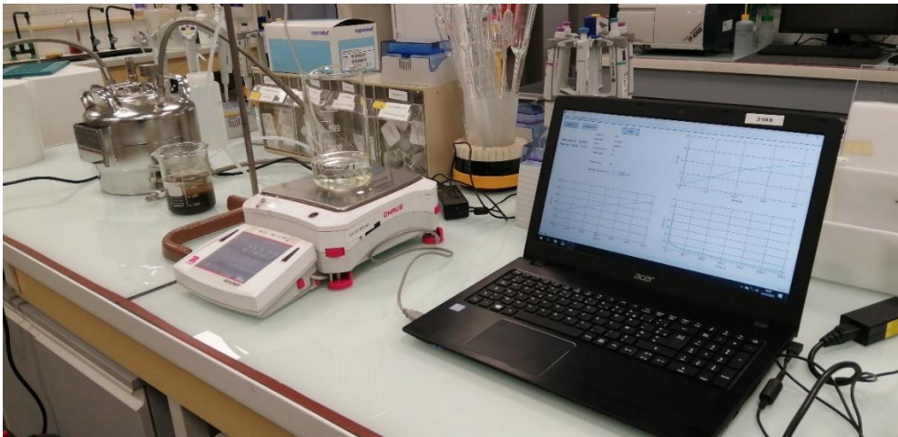
Fig. 7.10: Experimental setup for measurement of specific cake resistance
