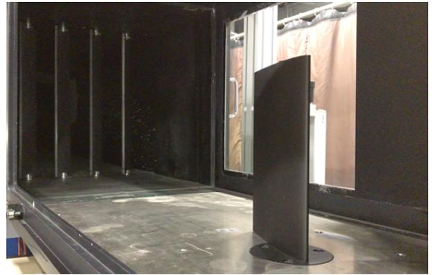
Figure 1: The experimental set-up showing the wing model at incidence and the array of louvre-door downstream.
