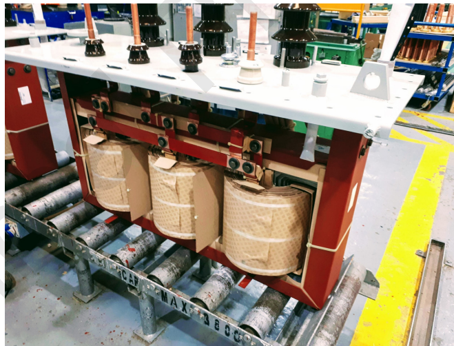
Figure 1: Picture of the distribution transformer in the production line at Tadeo Czerweny S.A., Argentina. View of the windings, magnetic core, current bars and steel frame.
