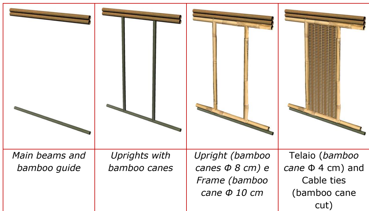
I.67 Assembly diagram of the technological panels
