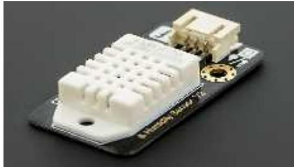
Gambar 4. DHT22 Sensor Suhu dan Kelembaban (Wijaya, 2016)
