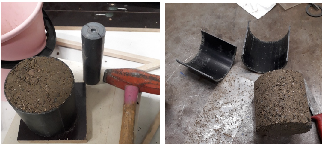
Figure 7-7. Compacted sample in the mould and released from the mould with required dimensions for hydraulic conductivity testing.
