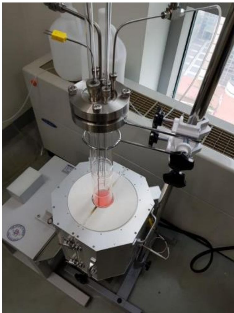
Figure 2.5. Optical image of electrochemical system for \text{SiO}_2 reduction in \text{CaCl}_2 molten salt.
