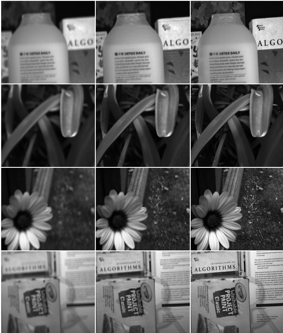
Fig 4.1: Visualization of the proposed defocus deblurring method. The first column is the blurry image, second is the restored image, and the last column is the ground-truth image.
