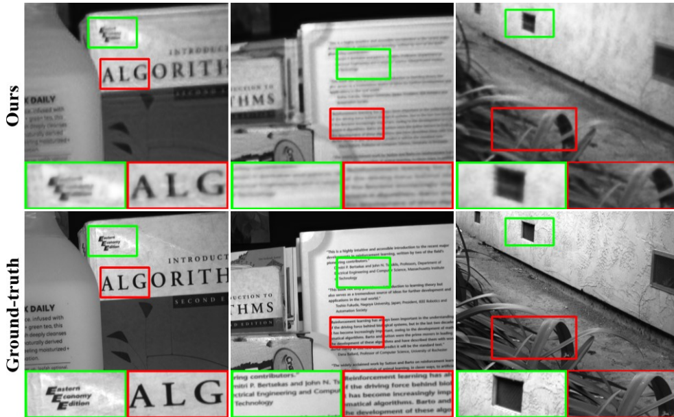
Fig 4.2: We compare with supervised methods [2, 3, 11] on the Google Pixel dataset. The first row is the blurry image and the last row is the ground-truth image. Our method shows less failure in defocus deblurring compared to other supervised methods.
