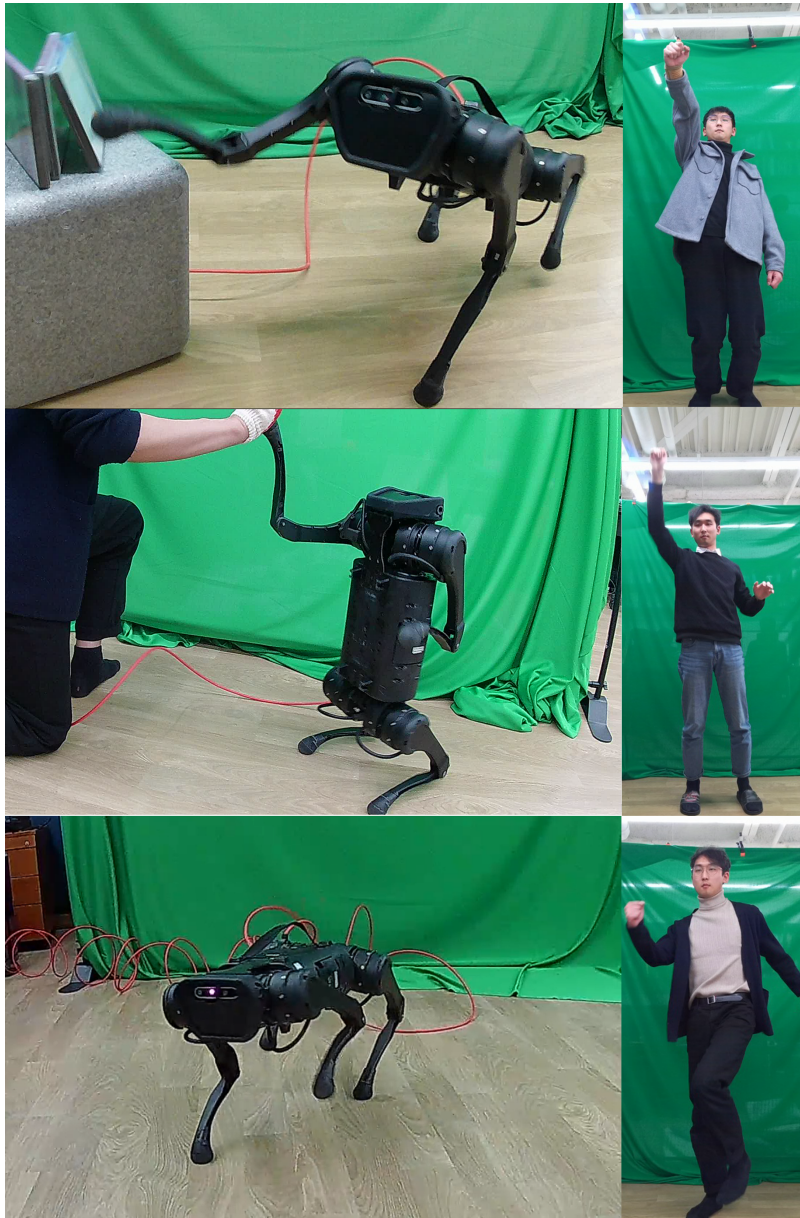
Figure 1.1: Novel control system that allows an operator to control a quadrupedal robot on various tasks.
