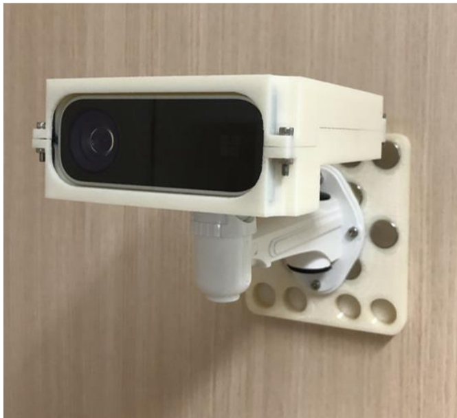
Figure 2.3: Azure Kinect DK with housing installed
