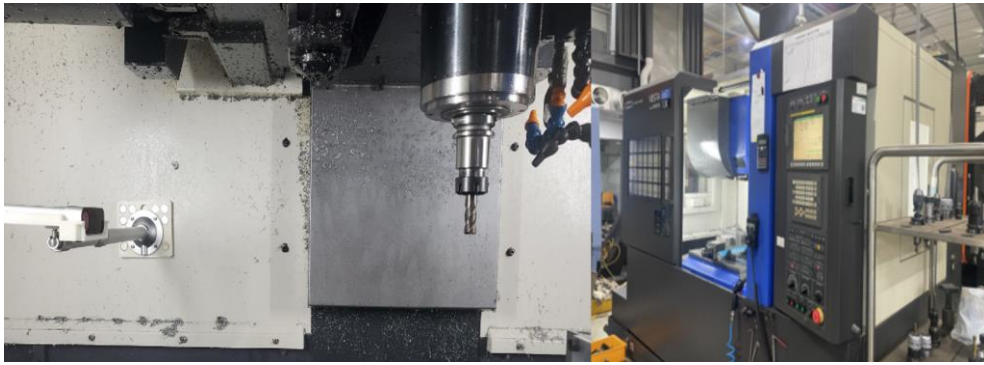
Figure 2.4: Attachment of packaged LIDAR into HSM-560A CNC
