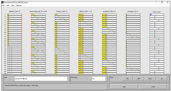
Figure 10. Determination of TDGC on six gas input data using the rule viewer on Transformer 6
