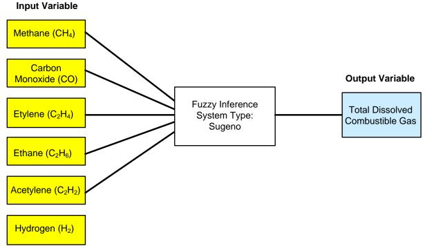
Figure 4. Model of fuzzy inference system-Sugeno
