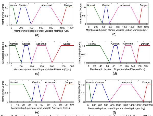
Figure 5. Complete membership functions for gas input variables respectively i.e. (a) Methane (CH<sub>4</sub>), (b) Carbon Monoxide (CO), (c) Ethylene (C<sub>2</sub>H<sub>4</sub>), (d) Ethane (C<sub>2</sub>H<sub>6</sub>), (e) Acetylene (C<sub>2</sub>H<sub>2</sub>), and (e) Hydrogen (H<sub>2</sub>)
