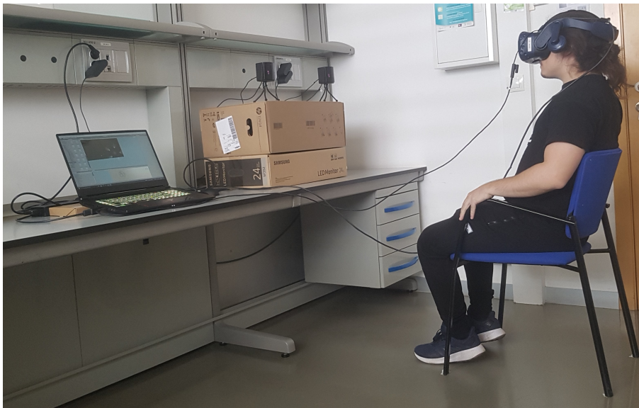
Figure 3.3: Experiment setup. The participant sits in a non-swivel chair, wearing the virtual reality headset and approximately one meter from the tracking sensors.
