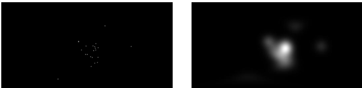
Figure 4.2: Example of the conversion process of a fixation map (left) to a saliency map (right). A Gaussian filter with a horizontal radius that scales to account for the distortion introduced by the equirectangular projection is applied to the fixation map.
