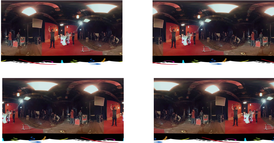
Figure 4.4: Example frame of a video augmented using longitudinal shifts. The original frame (top-left) is shown along with longitudinal shifts of 90° (top-right), 180° (bottom-left) and 270° (bottom-right).
