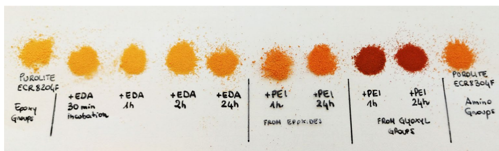
Figure 8. Picrylsulfonic acid assay of Purolite resin, which was previously functionalised in several manners.
