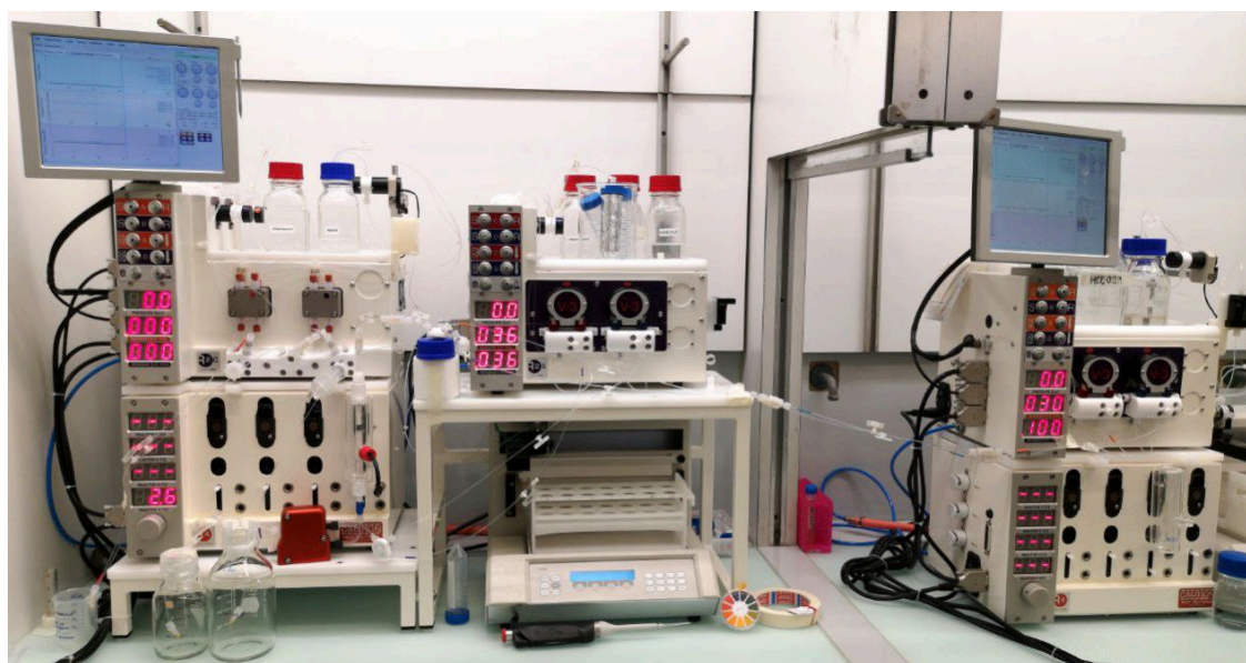
Figure 23. Set-up of the flow system for the 24 hours productivity test. Four peristaltic pumps were used for the purpose, two with the substrates (left) and two with the in-line separation process (HCl and EtOAc, on the right). The Zaiput separator is the red apparatus next to the packed bed reactor. Two bottles are placed at the downstream process for the collection of the two distinct phases.
