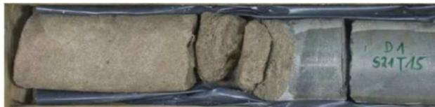
Figure 5: Sharp transition between the jet column and the soil.
