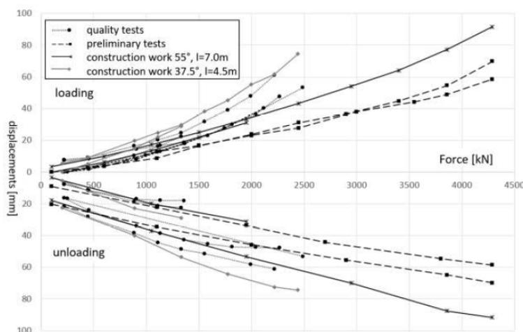
Figure 7: load-displacement-curves of selected jet grouted tie-back piles
