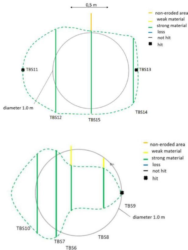
Figure 4: Determination of diameter by core drillings (above: near top of column, below: near base of column).
