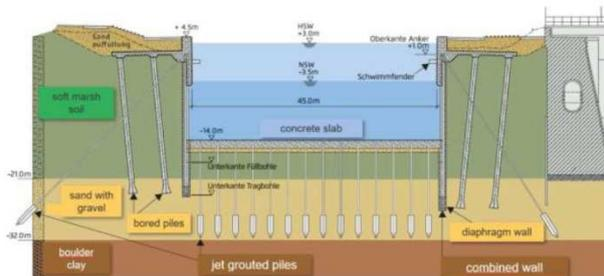
Figure 2: Cross section of lock chamber (schematic).
