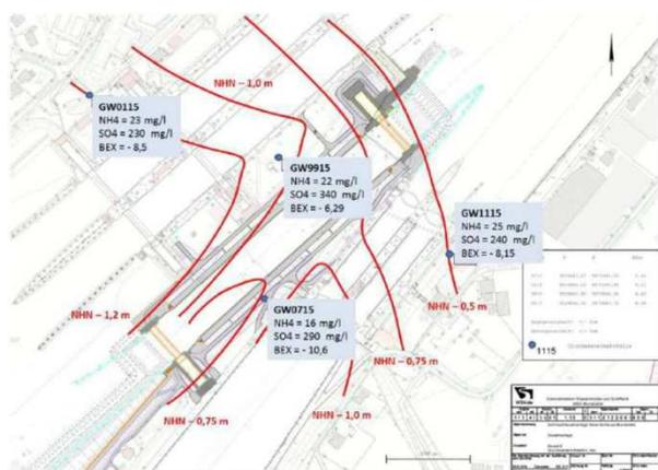
Figure 3: Groundwater contour plan with substance concentrations (statue 2015).
