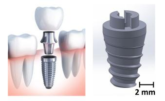
**Figure 1.** Left: Schematic picture of components in a simple dental implant consisting of (from the top): Crown, Abutment, Strut [5]. Right: CAD drawing of simplified combined strut and abutment.
