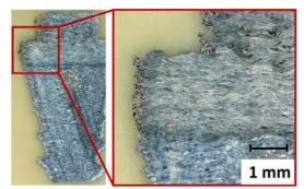
**Figure 2.** Sample shown as cut, embedded, polished and etched. Different material compositions visible for the lower and top part.
