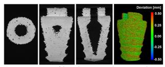
Figure 3. X-Ray CT scan of the implant specimen showing X, Y and Z cross section projections and part deviation plot from the nominal CAD model.
