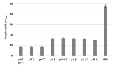
**Fig. 3** Protein recovery efficiency from *C. vulgaris* at various pH values. The algae suspension (5  $g_{DW}$ ·k $g_{SUS}^{-1}$ ) was PEF treated (40 kV·cm<sup>-1</sup>, 1 µs, spec. energy of 150 kJ·k $g_{SUS}^{-1}$  means 8.4 kWh·k $g_{DW}^{-1}$ ) and afterward incubated for 24 h at room temperature under the influence of different pH values in water or leftover medium conditioned to defined pH values
