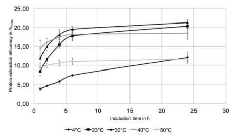
**Fig. 2** Time course of protein recovery efficiency after PEF treatment of *C. vulgaris* in dependence of incubation temperature. The microalgae suspension  $(5 \text{ g}_{DW} \cdot \text{kg}_{SUS}^{-1})$  was treated with a specific treatment energy of 150 kJ·kg<sub>SUS</sub><sup>-1</sup> and then incubated at different temperatures (Figure: Scherer et al. (2019))
