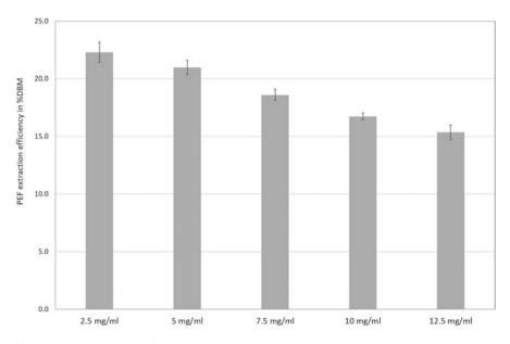
**Fig. 4** Protein recovery efficiency from *C. vulgaris* in dependence of biomass concentration. *C. vulgaris* suspensions were PEF treated (40 kV·cm<sup>-1</sup>, 1  $\mu$ s square pulses, 150 kJ·kg<sub>SUS</sub><sup>-1</sup>) and incubated for 24 h at room temperature (Figure: Scherer et al. (2019))
