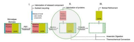
Fig. 1 Biorefinery concept based on PEF technology in which all biomass fractions are used efficiently
