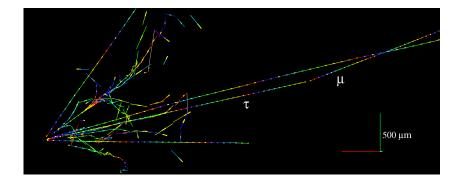
**Figure 43.** Event display of a simulated  $\nu_{\tau}$  event in the FASER $\nu$  emulsion detector. Reproduced from [393]. CC BY 4.0.
