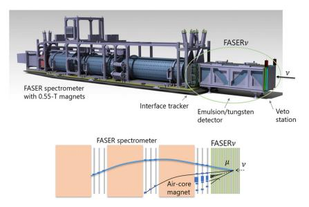
**Figure 35.** Sketch of the FASER detector. Reproduced with permission from [416]. CC BY-NC-ND 4.0 (top) and the topology to be seen in the interface tracker (IFT) and the FASER spectrometer [417] (bottom).
