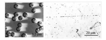
**Figure 59.** Left: halide bromide crystals (0.2  $\mu$ m linear size) seen under an electron microscope. Right: the track left by a minimum ionizing particle (10 GeV  $\pi^-$ ) in an emulsion film. Compton electrons are also visible on the right-bottom of the view.
