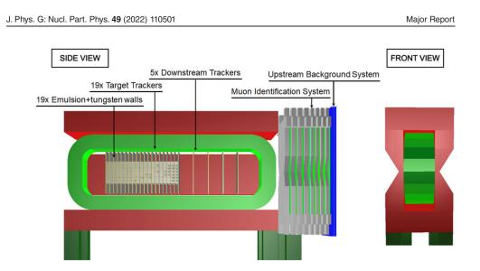
Figure 23. Schematic layout of the SND. Reproduced from [323]. CC BY 4.0.
