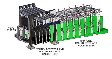
**Figure 37.** SND detector layout: the veto system is located upstream of the tungsten target, interleaved with emulsion and SciFi planes. Downstream of the target, 8 iron walls are followed by scintillating stations with the function of an hadronic calorimeter and a muon identification system.
