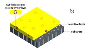
Fig. 8. Schematic diagram of AQP membrane configurations a) AQP supported lipid bilayers (SLBs) embedded in a thin active membrane layer and b) AQP vesicle immobilized within a dense membrane active layer (Tang et al., 2015) with copyright permission from Elsevier.
