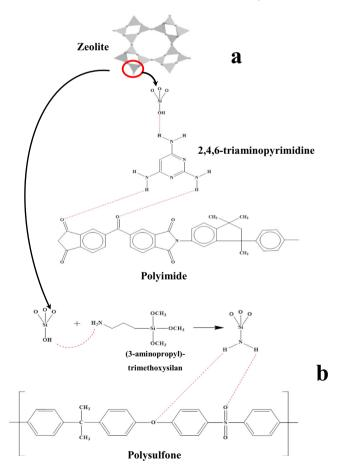
**Fig. 5.** Zeolite binding sites with polymeric membranes through: (a) application of compatibilizer and (b) zeolite conditioning. The figure was constructed based on the information presented in (Muntha et al., 2018; Yong et al., 2001).
