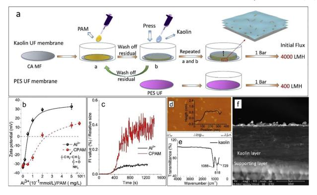
Fig. 4. 2 D kaolin membrane synthesis and characterization as reported in (Liu et al., 2019): (a) preparation steps; (b) zeta potential with two cross-linking agents (c) flocculation index of the two cross-linking agents; (d) Atomic force microscopy (AFM) analysis (e) FTIR-ATR spectrum of kaolin; (f) Scanning electron microscopy images of the produced membrane.
