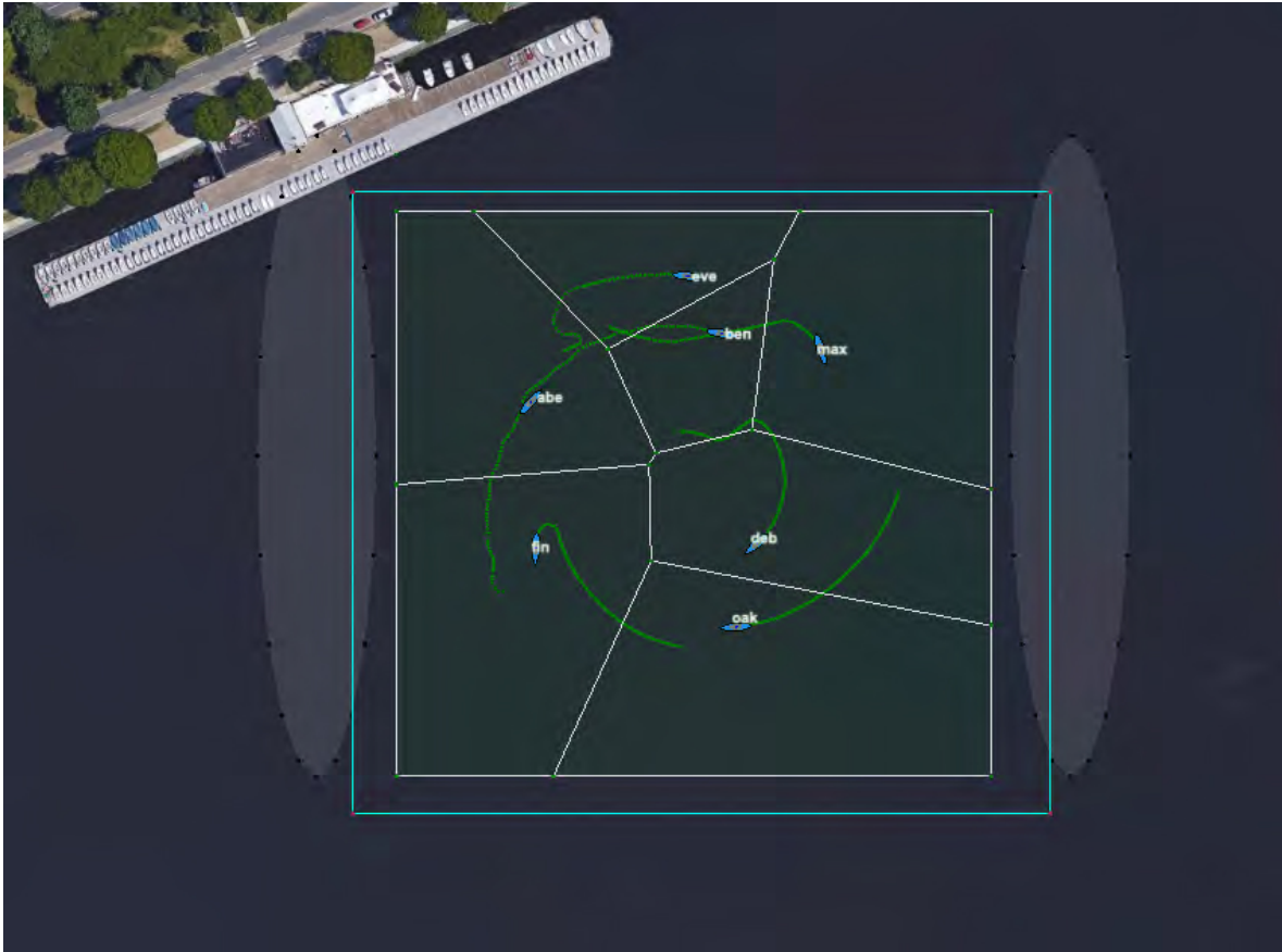
Figure 4.44: Vector field and Voronoi behavior operating on the Heron USVs as seen from pMarineViewer during the hardware test. The inner square region is the established 150m by 150m cover region. The Outer square region is the operational safety boundary established for the hardware test. The east and west ovals are the start and finish regions for the simulated adversary vehicle.
