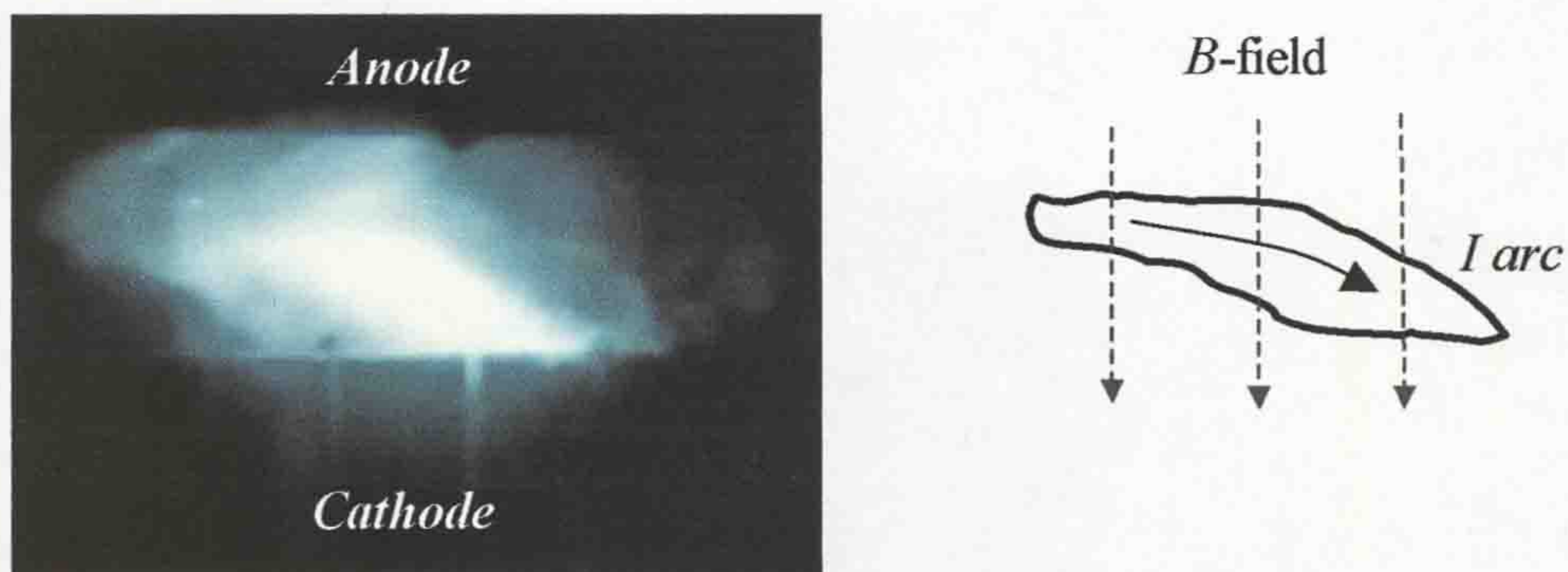
Figure 6.2 Photographic evidence demonstrating the existence of horizontal circular arc shape in the rotary arc current interrupter head (at 12.4ms, fig. 5.38b)
