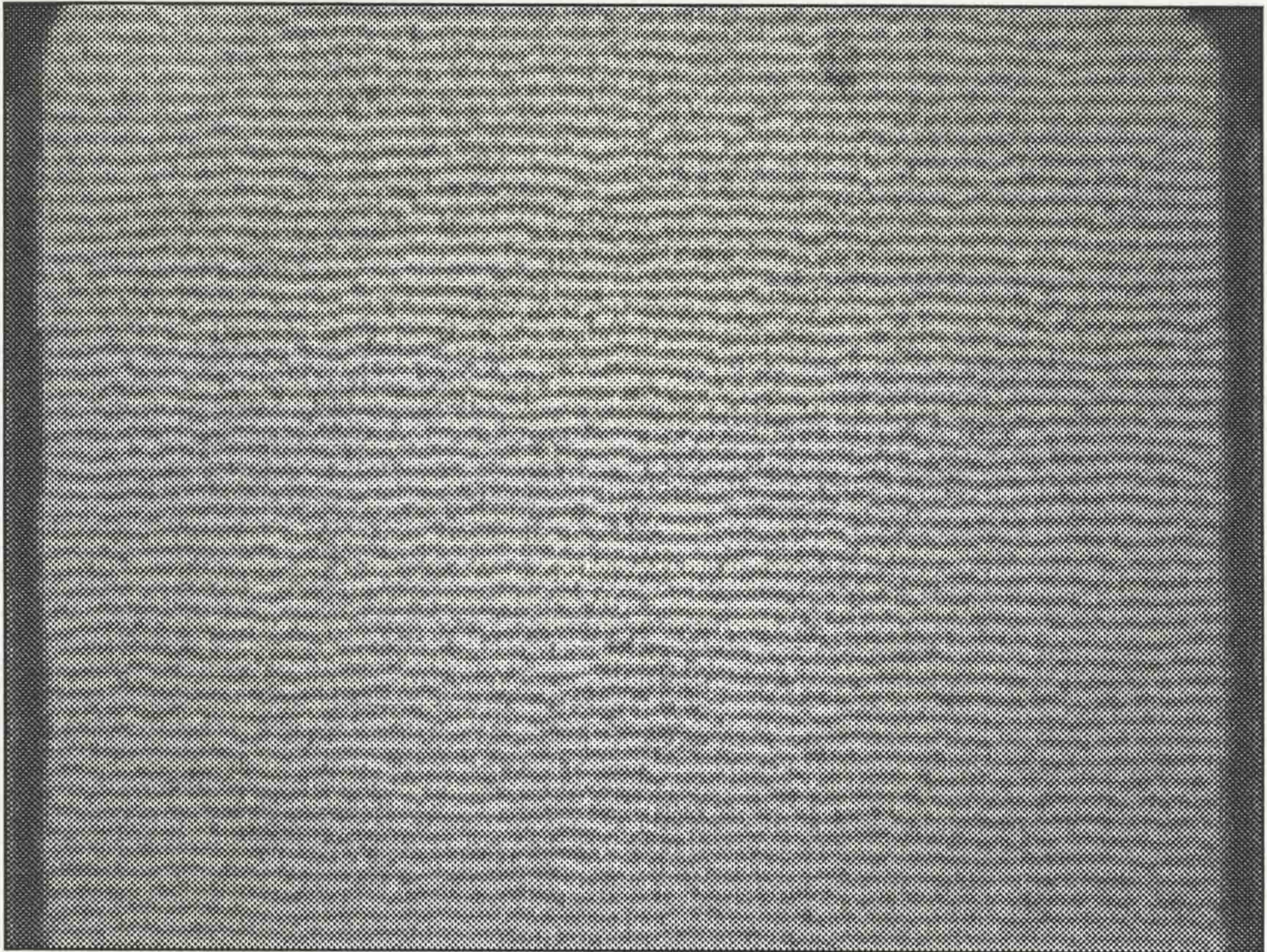
Image 7.12 (a) - The output from the coherent bundle when transmitting the test pattern for bit 1 (Numbered 0 to 7)
