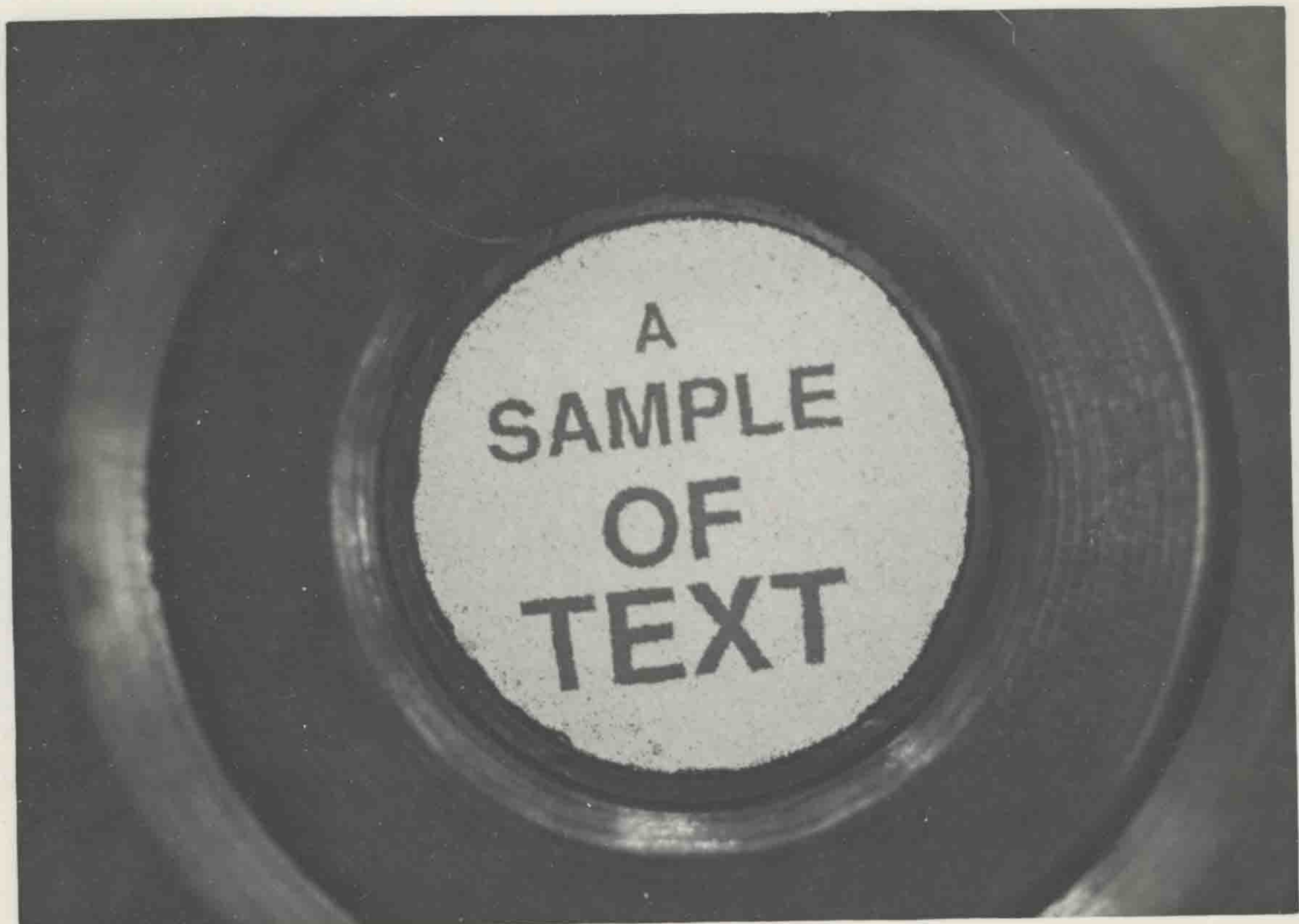
Plate 7.3 - The Output of a Coherent Bundle when Transmitting Text
