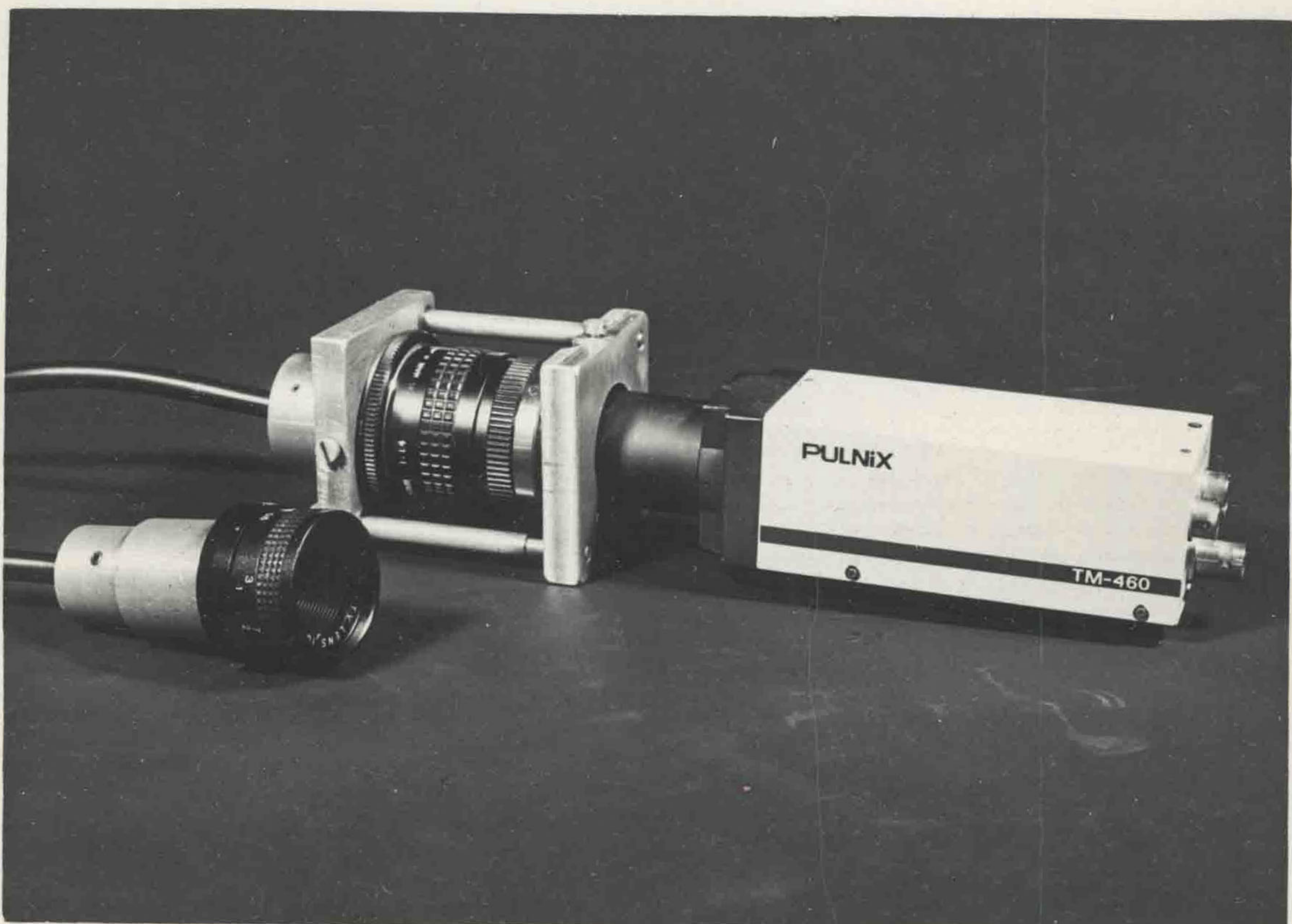
Plate 4.3 - The Camera and Lens Systems for Image Transmission
