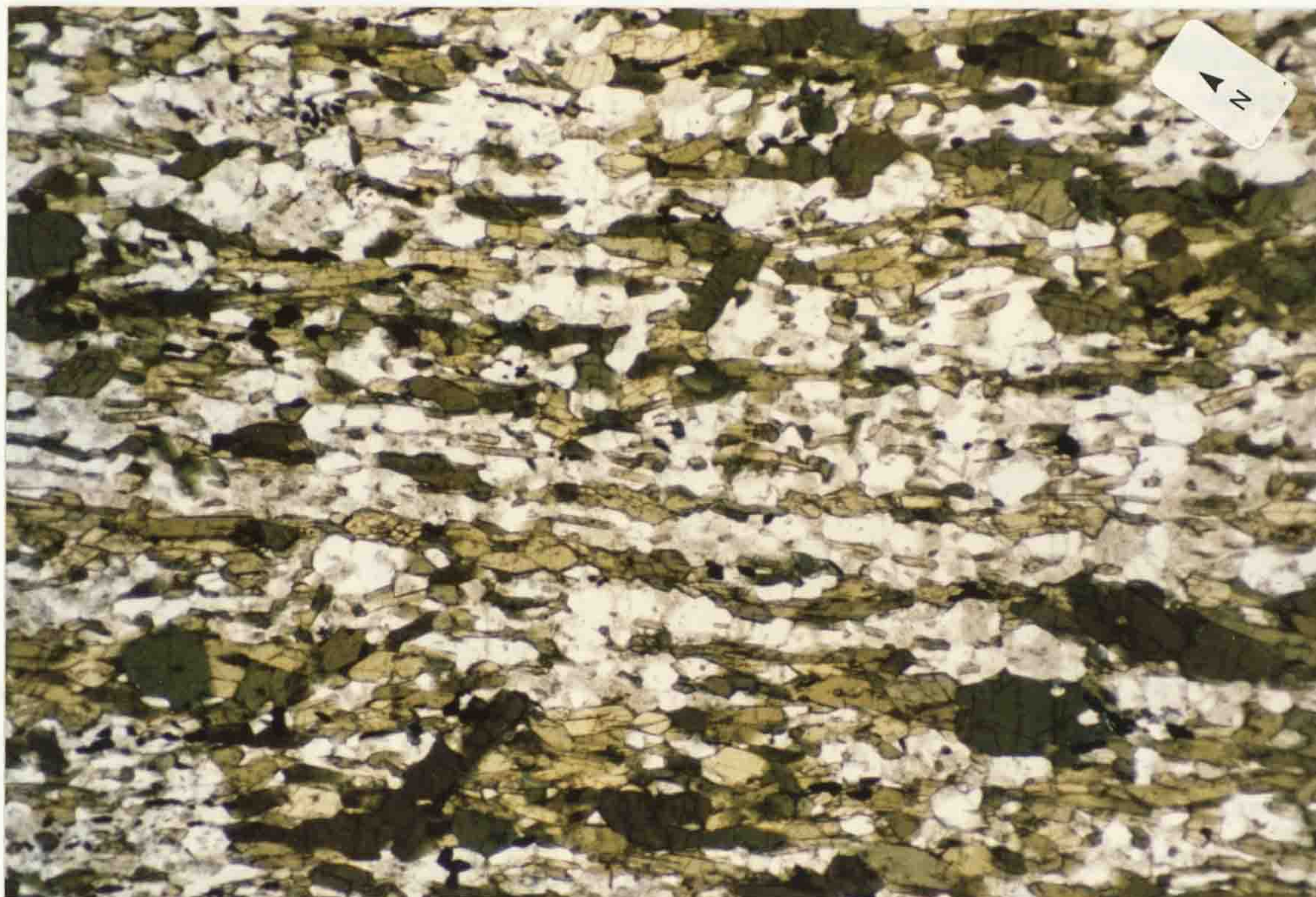
Figure 3.2: Segregated S_2 fabric in Lakes Marble amphibolite (X 29) PPL.
