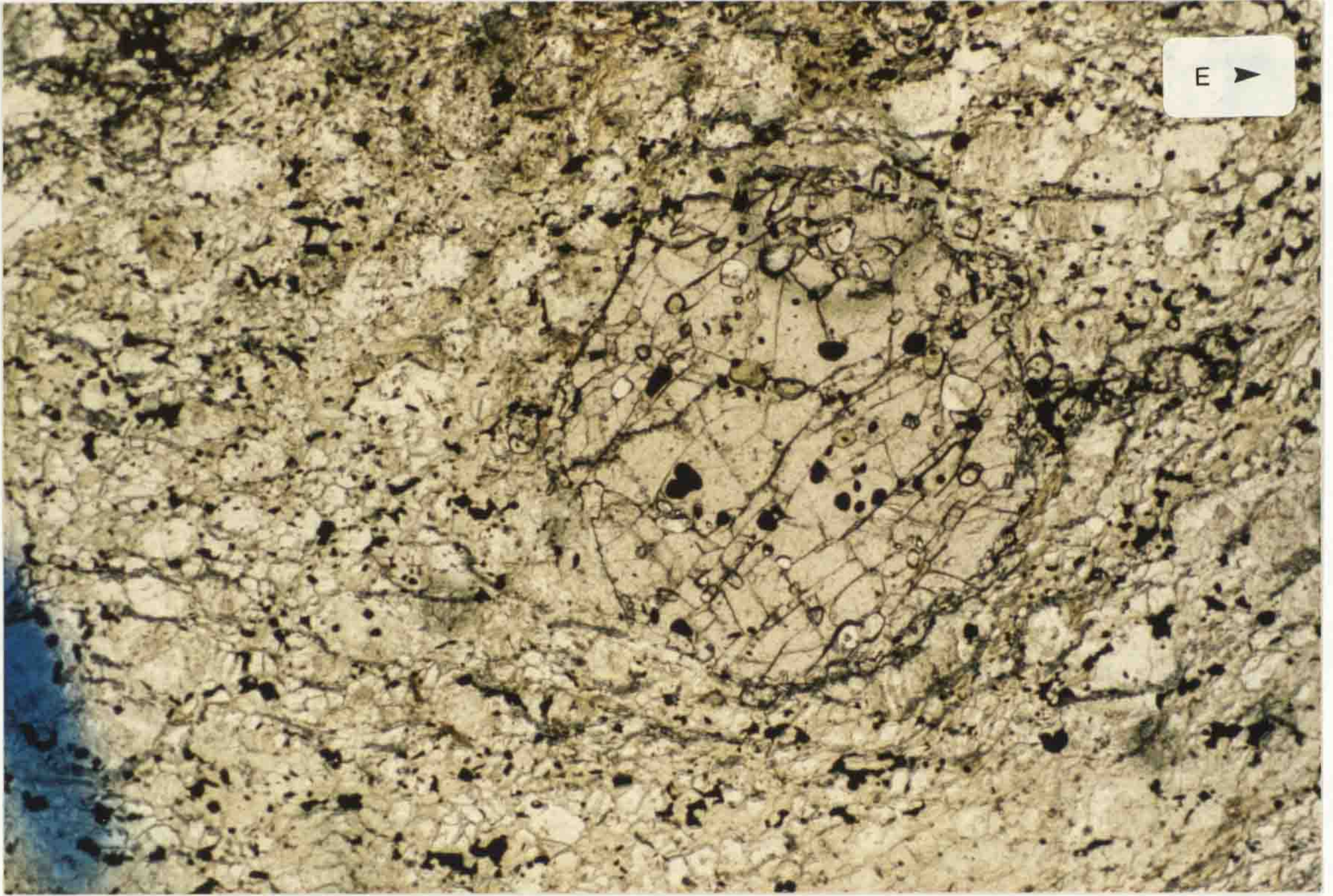
Figure 4.4: Contact aureole garnet containing rounded, xenoblastic inclusions (X 29) PPL.
