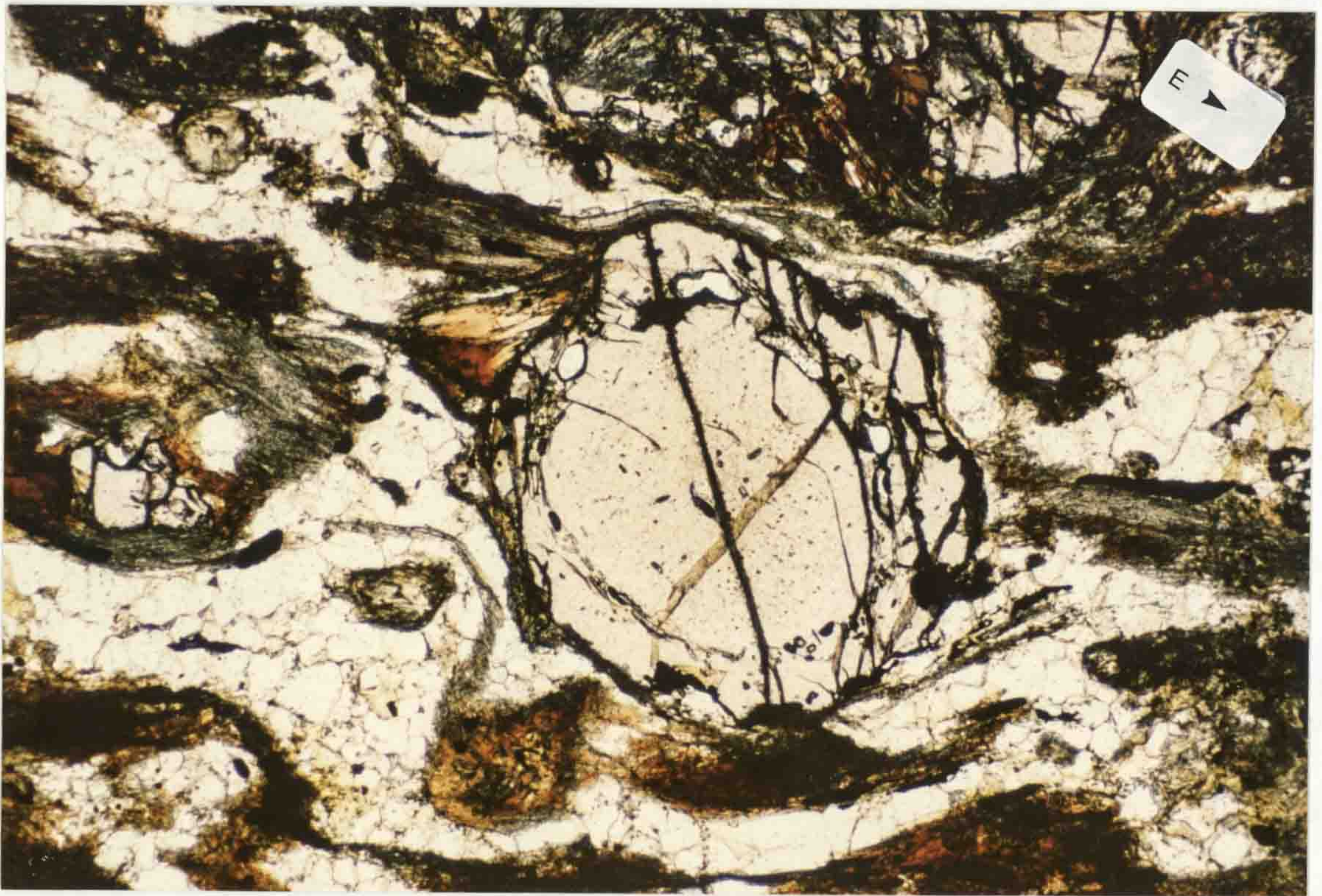
Figure 4.5: Contact aureole garnet with 'spherical' inclusion trail (X 29) PPL.
