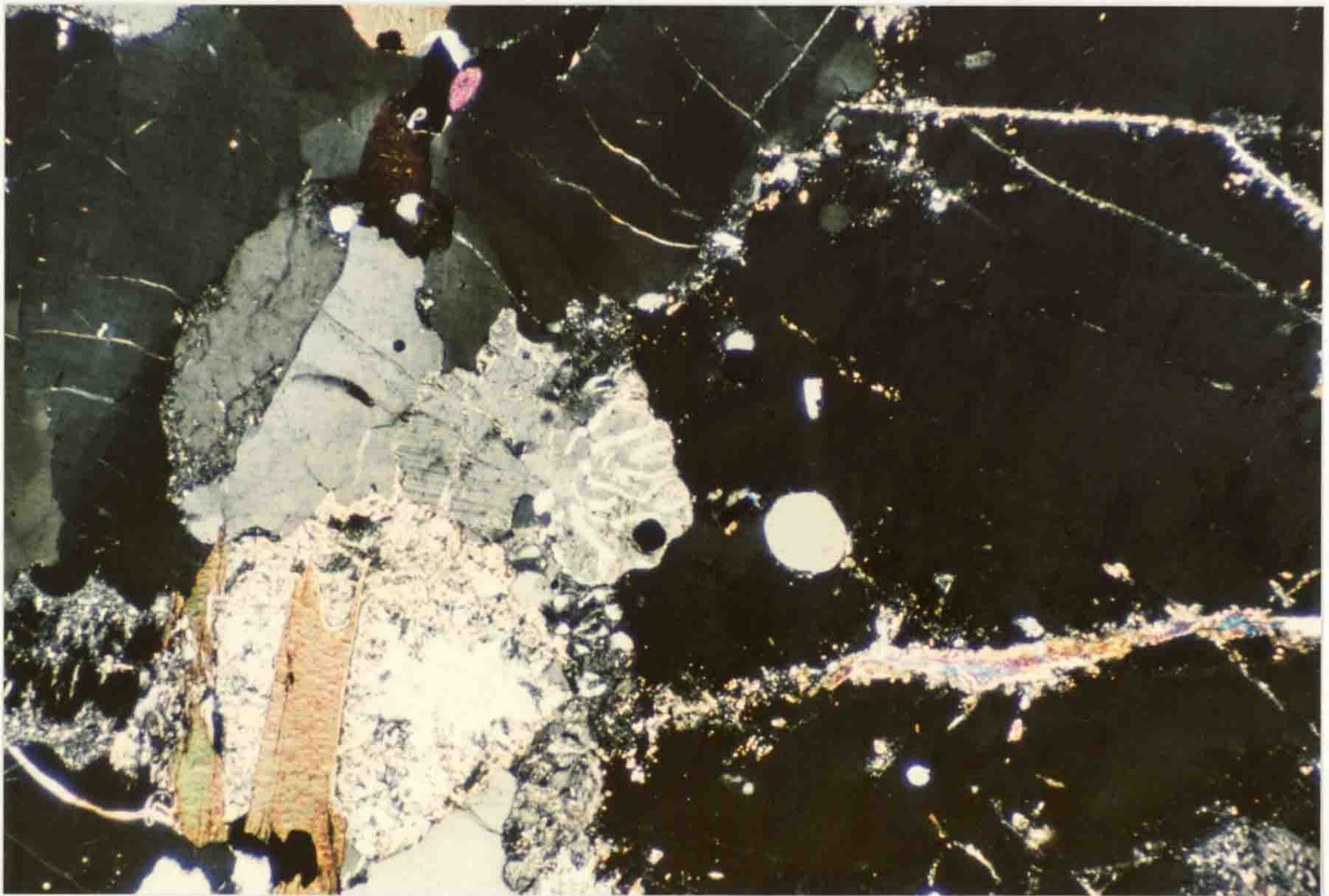
Figure 4.40: Myrmekitic intergrowth of plagioclase feldspar and quartz in contact aureole lithology (X 56) XPL.
