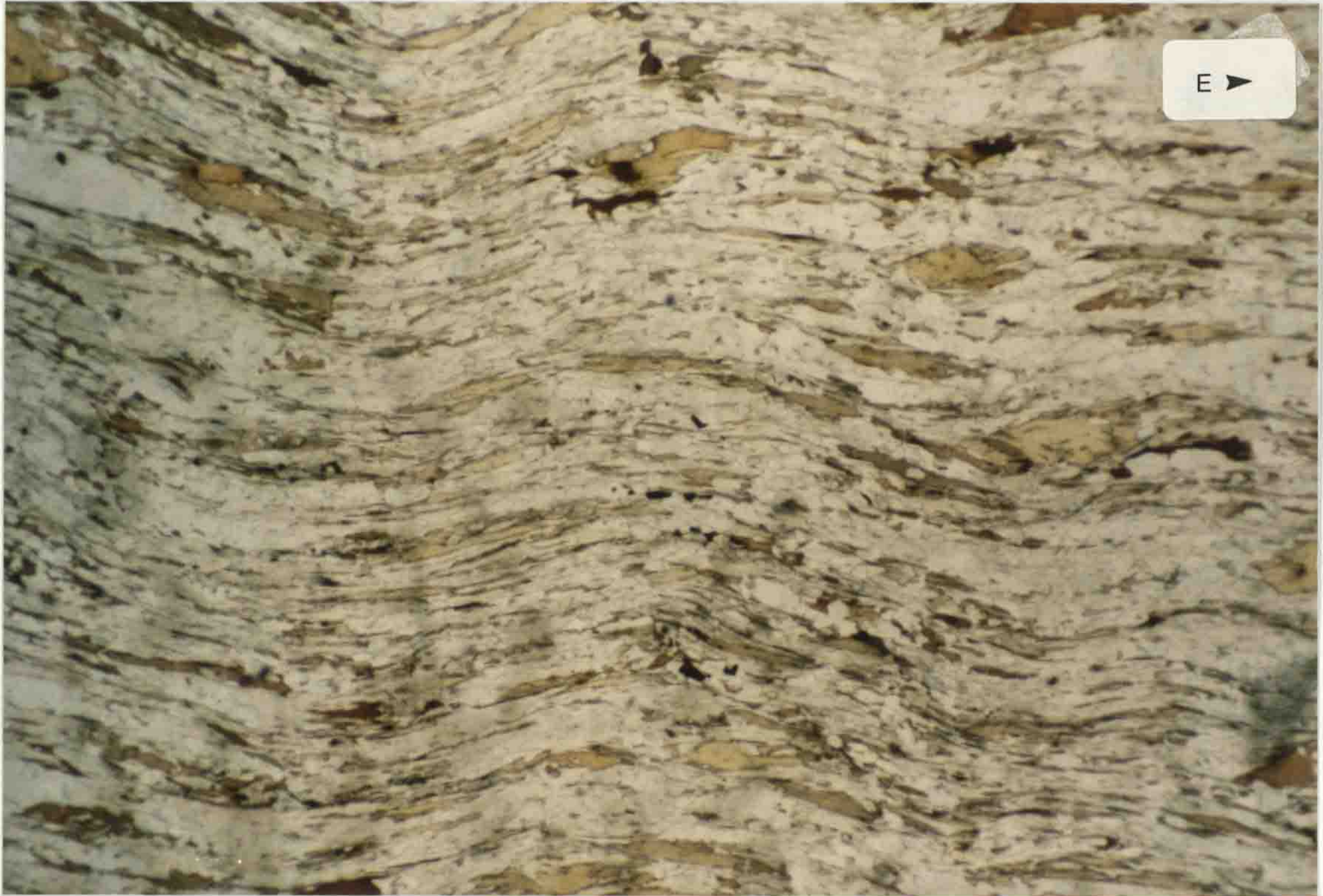
Figure 3.4: Gentle D_3 crenulation deforming S_2 foliation in Streamstown Formation pelite (X 29) PPL.
