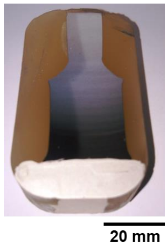
Figure 4-22: Photograph of LPBF in-situ shelling canister cross-section mounted in resin.
