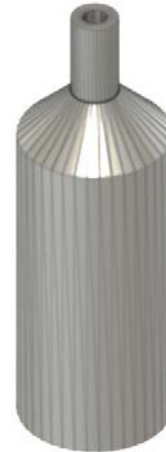
Figure 9-6: a) Solid impeller with centre aspect removed; b) simple canister to replace centre of impeller.
