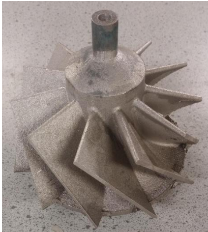
Figure 9-5: Completed LPBF shelled impeller following further CAD modifications: a) front view; b) bottom view with region of surface connected defects highlighted with red shading.
