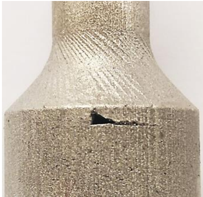
Figure 8-1: Hole in the side of LPBF canister with wall thickness 1.5 mm.
