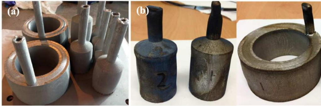
Figure 2-2: Photographs showing several canister designs (a) before and (b) after HIPing. Taken from [12].
