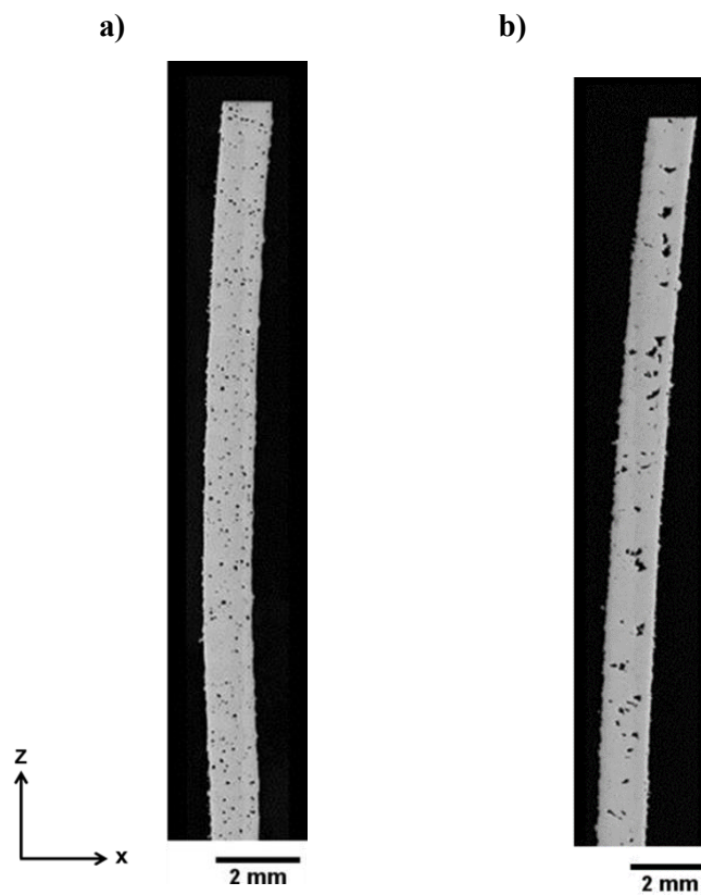
Figure 7-5: micrographs of XZ cross-section of walls with high area fractions of porosity. a) keyhole porosity in wall built with 40 \mu\text{m} layer thickness; b) LoF porosity in wall built with 60 \mu\text{m} layer thickness.
