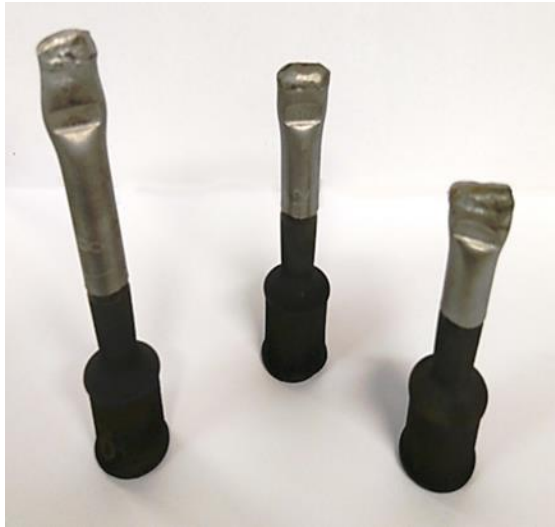
Figure 8-3: In-situ shelling canisters after being removed from the HIP.
