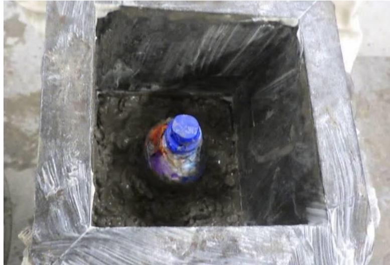
Fig. 4. Ecobrick placed centrally in concrete cube casing.
