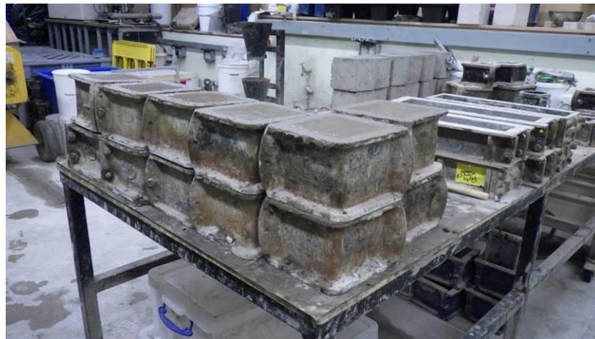
Fig. 5. Casted Concrete Cubes.
