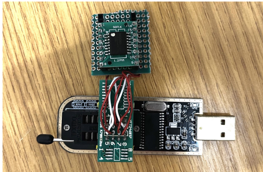
Figure 3: Dumping BMC firmware with a flash programmer.
