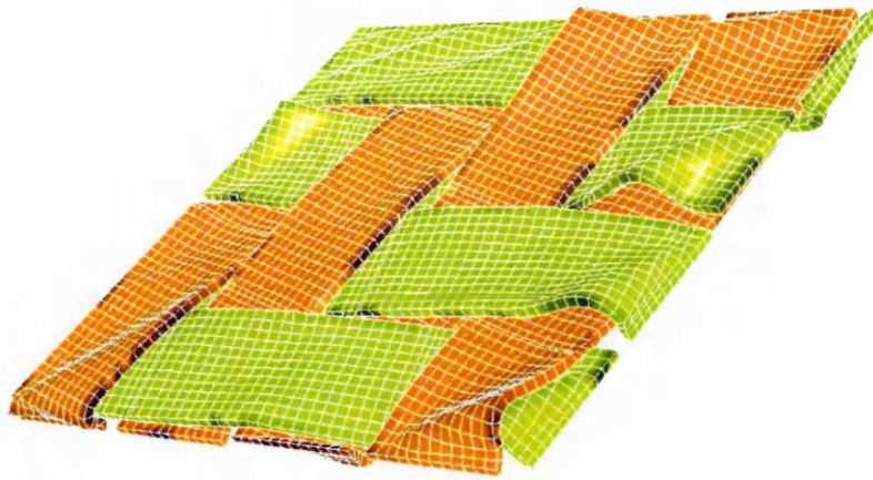
Fig. 8.1. 2/2 twill unit cell representation
