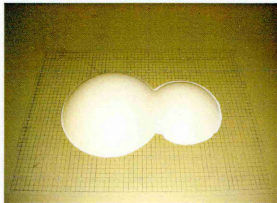
Fig. 4.8 The double hemisphere mould, placed upon the metal vacuum forming plate
