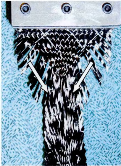
Fig 6.2. 2/2 twill separation during bias extension testing (Arrows denote the direction of observed fibre separation movement)
