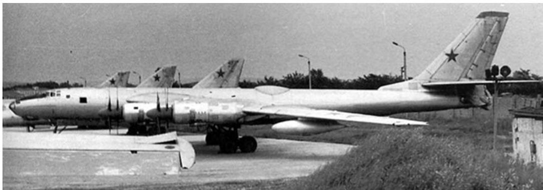
Figure 2-8 Tupolev Tu-95LAL nuclear test-bed airplane [54]
