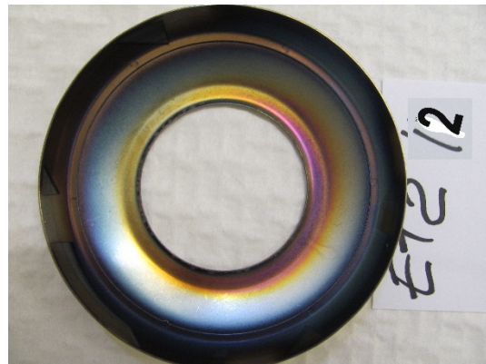
Figure 2. Bottom face of electrode 12 (last) in unit 19, acceleration tube 2 after over 40 years of operation.
