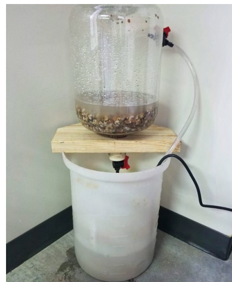
Figure 1: Example of the pump-included hydroponic wastewater system.
