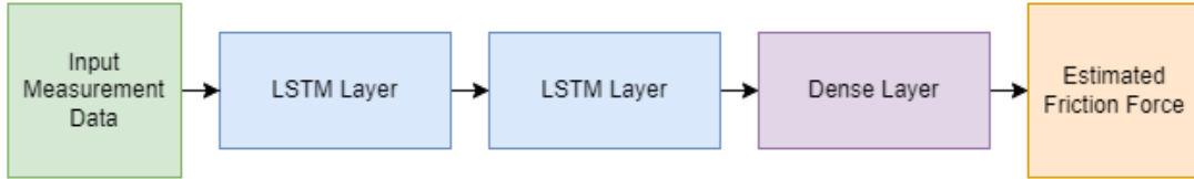
Figure 3.14: LSTM Network Architecture Layout for Friction Estimation on Inverted Pendulum System
