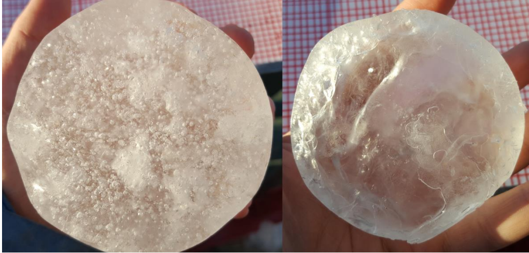
Figure 2.3 Difference between air inclusions for snow ice (left) and clear ice (right).
