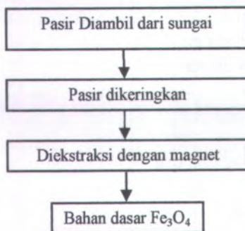
Gambar 3.1 Prosedur preparasi  $\text{Fe}_3\text{O}_4$
