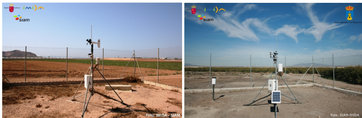
Figure 3. Example of the ground-based meteorological stations (Source: SIAM-IMIDA [47]).
