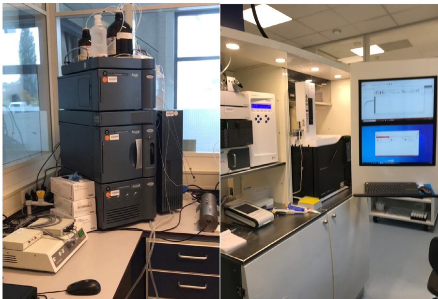
Fig. 5 QC area with typical UPLC equipment (left), and combined HPLC, GC for residual solvents, endotoxin and osmolarity equipment (right). The latter equipment is feasible to perform the QC before and after release for administration in humans.
