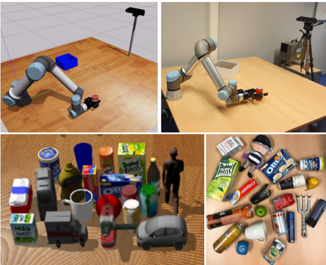
Fig. 8. Our experimental setups: ( top-left ) simulation environment in Gazebo; ( top-right ) real-robot setup. The pose of the robot and the camera in the simulation are consistent with the real-robot setup. ( bottom-left ) Objects used in simulation experiments; ( bottom-right ) Objects used in real-robot experiments.
