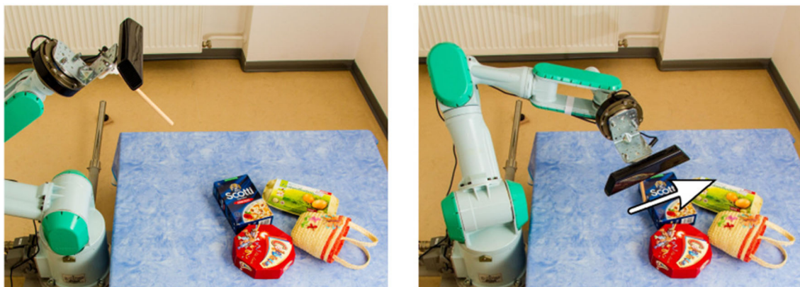
Fig. 6 Examples of active object segmentation in pile of objects scenarios: ( left ) The robot observes the scene, obtaining a point cloud from one perspective. ( right ) The robot decides to push the object from the bottom to segment them. The robot repeats these step to singulate all objects (adapted from [195])
