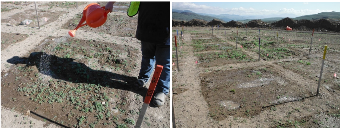
Figure 3.5: May and June watering of site preparation and seeding study at New Gold's New Afton Mine site. Watering was completed by hand using watering cans with dispenser heads (left). All plots were watered with 4\text{mm}/\text{m}^2 twice a week. The right figure shows a plot with standing water which was allowed to seep into the soil before more water was applied.
