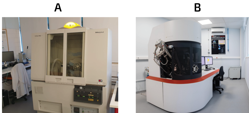
Figure 4.5: Characterization equipment used for the study of CuNPs-LIG composites. A) XRD and b) X-Ray Photoelectron Spectroscopy (XPS) equipment.
