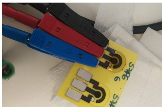
Figure 4.12: Connection established between the potentiostat and sensor. The cell cable connects to the WE, RE and CE on one end and the potentiostat cell cable connector on the other end.
