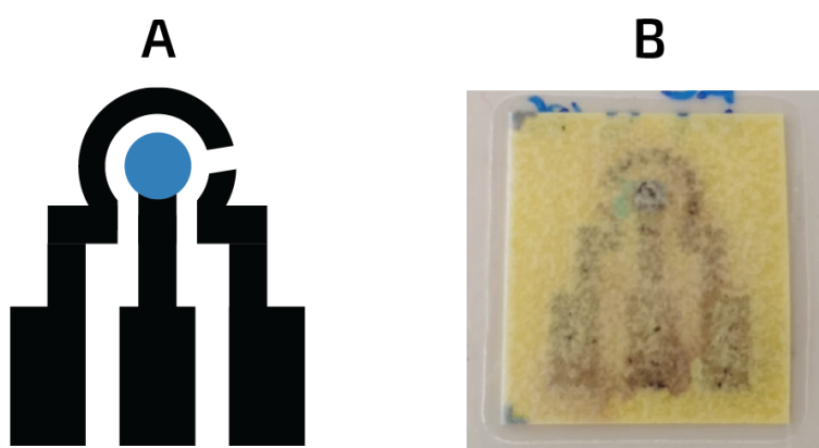
Figure 5.29: Sensor design for optimized laser parameters. A) In this image, black corresponds to the optimized laser parameters for LIG and blue refers to the CuNPs-LIG. B) Back of the sensor after CV experiments.
