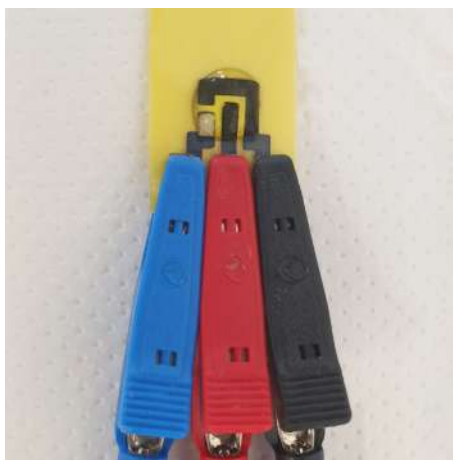
Figure 4.16: Sensor connection demonstration for electrochemical trials.
