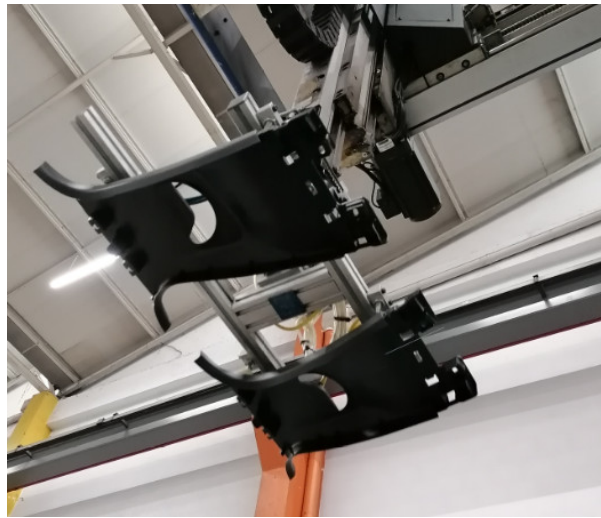
Figure 5. Three-axis robot responsible by taking the injected parts from the mould.
