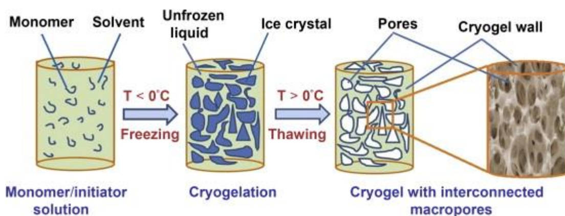
Figure 2.1. schematic representation of cryogel synthesis [151].
