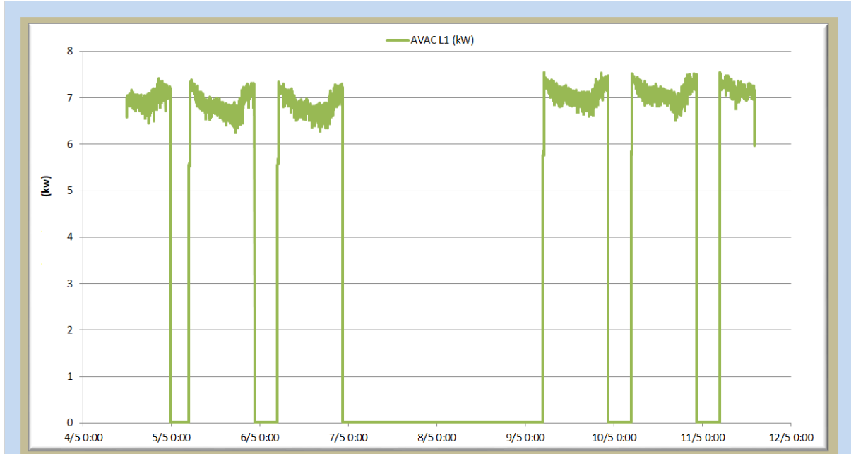
Figure 49: Load profile (kW) of UTAs Line 1 (integration step 1min)
