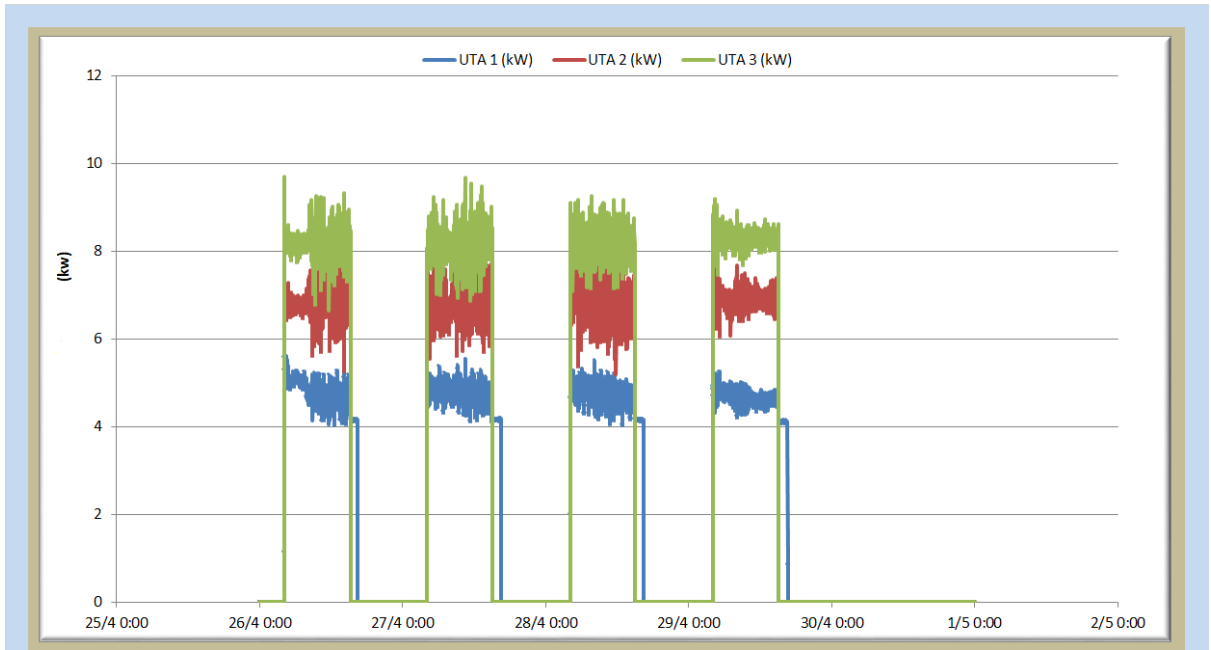
Figure 47: Load profile (kW) of UTAs Line 6 (integration step 1min)
