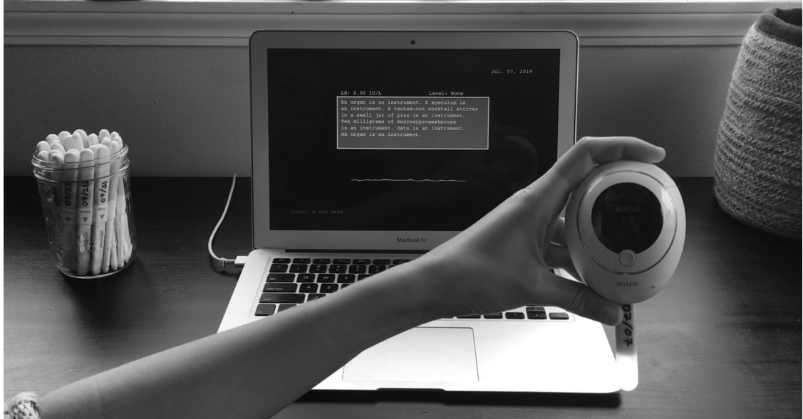
FIGURE 10.1 Reconfigured wands are inserted into a hacked Mira device to control the story on an adjacent computer screen. The screen also displays data, including the date of the original LH measurement, the concentration level, and a running graph scaled to “typical” LH fluctuations over a thirty-day cycle. Credit: Julie M. Funk.
