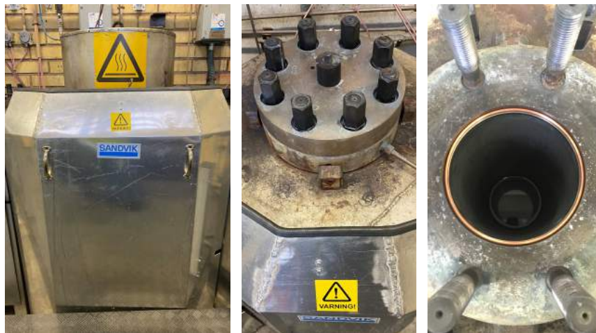
Figure 7-2: The PWR autoclave setup at Sandvik: the autoclave (left), the top without cover (centre), the inside (right).
