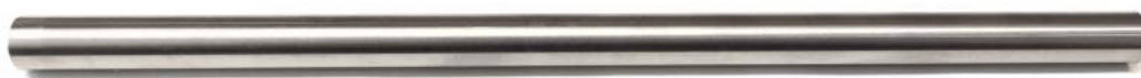
Figure 7-1: Photo of as-fabricated Cr-coated Optimized ZIRLO™ cladding sample (200 mm in length, 9 mm in diameter, wall thickness 0.6 mm).
