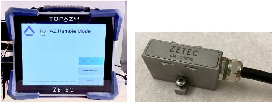
Figure 3.1: Data acquisition hardware unit, TOPAZ64 ® (left), and linear PA probe, LM-5MHz (right)
